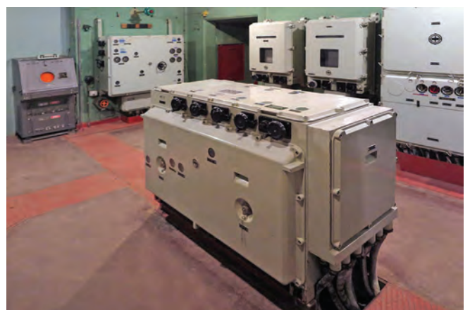
Artillery calculator within the Artillery Control Centre at Stevns Fort. This mechanical computer took many variables including temperature, wind, pressure and so on and coupled with the visual or radar plot of a target calculated elevation and heading to deliver an accurate trajectory
